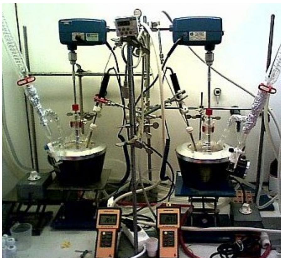
**Figure A.2.** Overview of catalytic test setup in fume hood. This setup was used for G1, G6, and G6IM heating programs.
